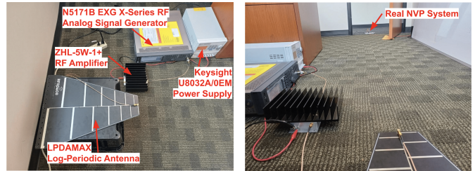
(a) Experimental setting for remote attacks (b) Remote attack outside of a room
